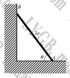
The figure above shows a uniform ladder AB of length 2a and of mass m resting with the end A on rough horizontal ground and the end B against a smooth vertical wall. The ladder is inclined at an angle  $\theta$  to the ground.
