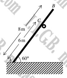
The figure above shows a uniform rod AB of length 8 metres and of mass 15kg. The rod is resting in equilibrium with the end A on rough horizontal ground and the point C, where AC = 6 metres, on a smooth peg. The rod is inclined at  $60^{\circ}$  to the ground.
