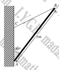
The figure above shows a uniform rod AB of length 5 metres and of mass 60 kg resting in equilibrium with its end A smoothly hinged on a vertical wall. A light string BC is attached to a point C on the wall which lies vertically above A, such that |AC| = |CB|.
