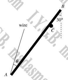
A non uniform rod AB of length 6 m and weight 600 N rests in equilibrium over a smooth peg at C, where BC = 1 m. A light inextensible wire is attached to the rod at A, and is inclined at an angle  $\theta$  to the rod. The wire and the peg support the rod at 30° to the vertical, as shown in the figure above.
