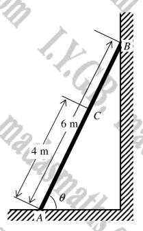
The figure above shows a ladder of length 6 metres and mass 20 kg, with one end A on rough horizontal ground and the other end B against a smooth vertical wall. The ladder is modelled as a uniform rod and lies in a vertical plane perpendicular to the wall and the ground, inclined at an angle  $\theta$  to the horizontal, where  $\tan \theta = \frac{4}{3}$ .
