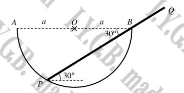
A smooth hollow hemispherical bowl of radius a and centre at O, is fixed so that its circular rim lies in a horizontal plane.
